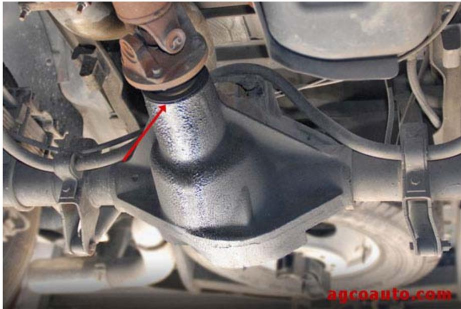
Closer inspection and from another angle reveals the true source of the leakage. The differential pinion seal is leaking oil, which is blowing back onto the rear cover. Simply replacing the cover seal would do no good. Replacing only the pinion seal can damage certain vehicles and also present a very dangerous situation.
